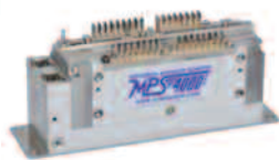
INTELLIGENT ETHERNET PRESSURE SCANNER
